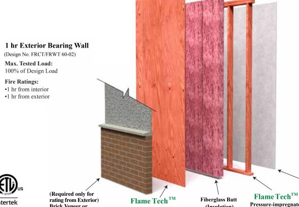
rating from Exterior) Brick Veneer or 3/4 inch Cement Plaster (stucco) (1 hr from exterior face)
